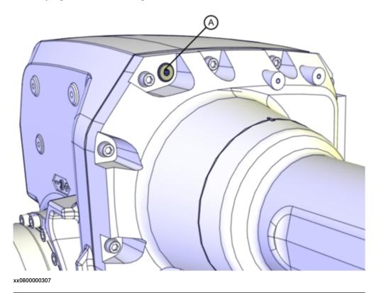
A Oil plug, for filling and draining
